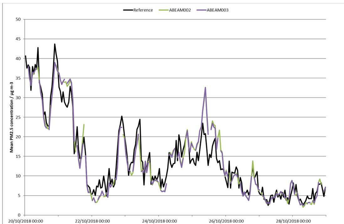
Figure 2: Time series chart of hourly mean sensor and reference PM<sub>2.5</sub> concentrations over the test period following application of scaling factors. ABEAM001 is excluded due to this sensor being defective.
